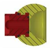
The "Quik-Change" Nozzle Tip is installed with a bayonet mount, and a simple 90° twist is all it takes to lock it into the ball. It is O-Ring sealed at the bottom and lip sealed at the top to prevent the mounting slots and tabs from becoming contaminated and difficult to disassemble.
