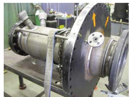
Steam-jacketed fabrication with three spray nozzles installed through the jacket.
