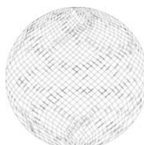
Orbitor 4 nozzle spray pattern
